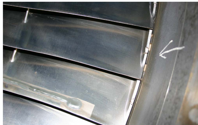
Fig. 11 The installed magnet can just be seen through the tip gap over the blade (see arrow)
